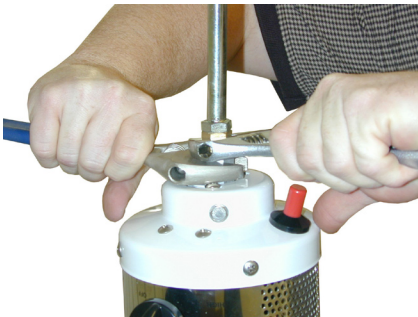
Figure 10 - Tightening Manifold and Burner Assembly
